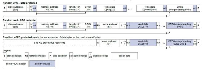
The memory address field sets the byte address of the first memory location to be read from or written to. Only 16-bit-word aligned reads/writes are supported, i.e. the LSB of memory address has to be zero always. The read/write data is transferred MSB first, low byte before high byte.
